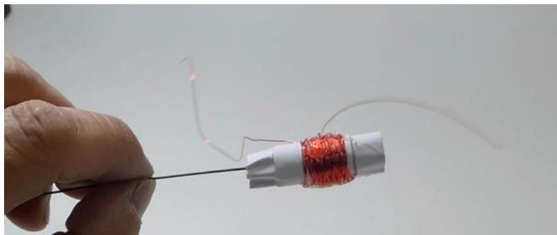
6. Secure the wound wire in place with hot glue.
