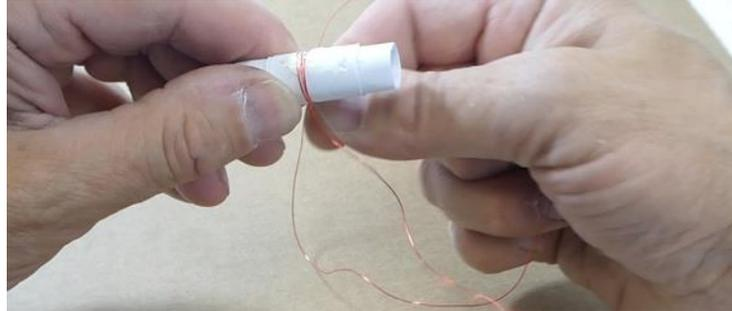
5. The area of wound wire should measure about .50"–.75" (long enough to cover the length of the magnet inside the paper roll).
