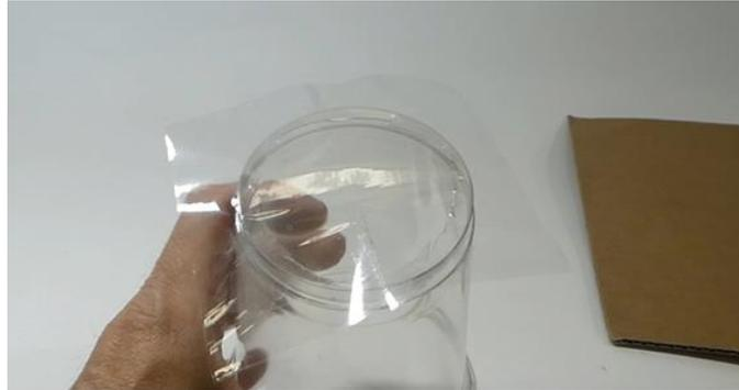
14. Glue the voice coil roll to the center of the circular cup base piece (plastic disc) that you cut out earlier.
