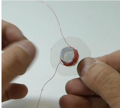
15. Apply a thin bead of hot glue around the edge of the underside of the plastic disc (on the opposite side of the disc from where the voice coil roll is glued).
