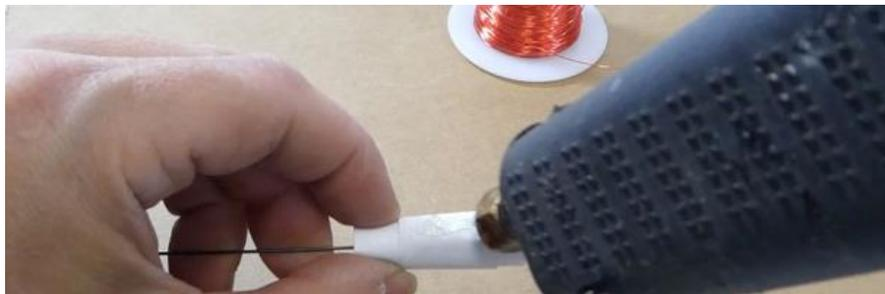
4. Making sure to leave a long, loose lead wire (4"–6"L), begin wrapping the wire around the paper roll (through the hot glue). Wrap 50 turns of wire around the roll. The wraps do not have to be really tight but should be firm.
